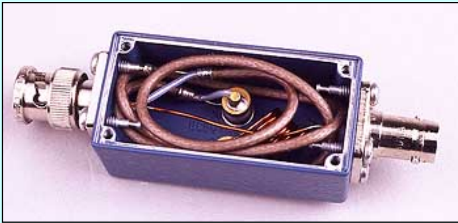
Figure A--This simple notch filter is easy to tune and uses available components.
