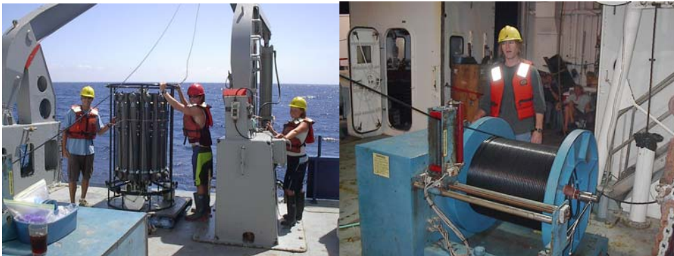
Figure 1. Sampling system currently in use for iron and aluminum on the CLIVAR Repeat Hydrography Program (C. Measures and W. Landing).
