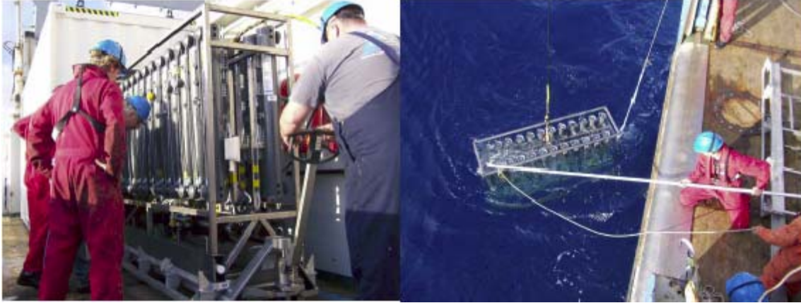
Figure 2. Rectangular, ultraclean titanium frame with 24 Go-Flo samplers (12 L) and CTD, etc. sensors in front of its own ultraclean laboratory van. Deployment with 20 mm Kevlar cable (9000 m on winch drum) with internal signal cables for sensors data transfer and for tripping bottles from deck at any desired depth. Pneumatics for closing samplers allows any shape frame (i.e., departing from circular shape prescribed by traditional stepping motor/trip wires). Upon recovery, the complete frame enters its clean container and samplers are emptied via filter cartridges into sample bottles. The system was successfully tested November 2005 in the Canary Basin, and will be used in IPY GEOTRACES 2007-2008 sections during Polarstern expeditions.
